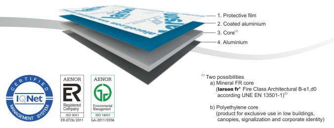
Aluminium composite panels for architectural wall cladding
